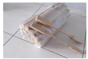
Figure 1: Dog bone shaped tensile test specimens
