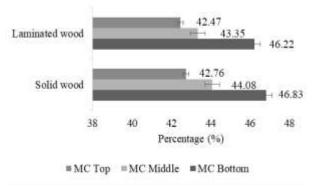
Figure 1: Moisture content for solid wood and laminated wood due to the different portion.
