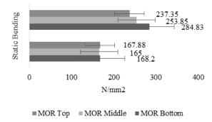
Figure 3: Modulus of rupture for static bending test on solid wood and laminated wood due to the different portion
