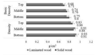
Figure 2: Density and basic density for solid wood and laminated wood due to the different portion
