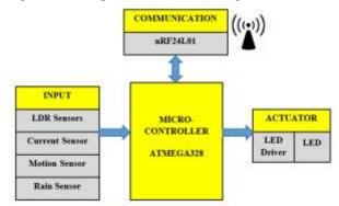
Figure 6: Design of the Mesh Client Node
