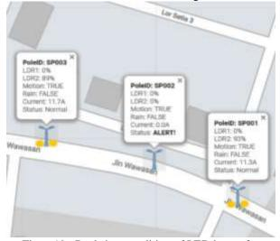
Figure 19: Real-time condition of LED lamps for maintenance purpose
