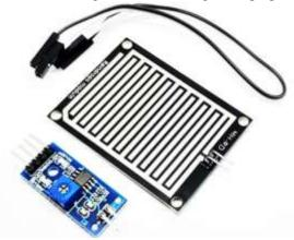
Figure 11: Rain/Water Sensor
