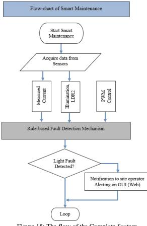
Figure 15: The flow of the Complete System Maintenance Mechanism
