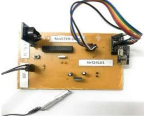
Figure16: The prototype of Mesh Master
