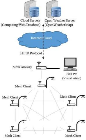
Figure 4: The layout of the wireless network communication and cloud connection
