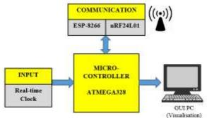
Figure 7: Design of the Mesh Master Node
