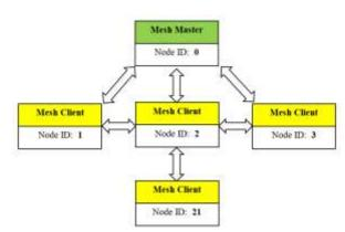
Figure 5: Interconnection of nodes in the mesh network
