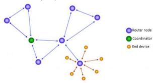
Figure 1: Wireless Sensor Network [11]
