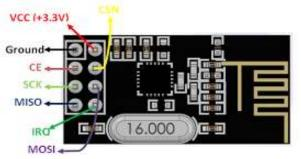
Figure 13: nRF24L01 wireless transceiver module
