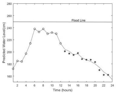
Figure 4: Comparison of the predicted and actual values of present water levels (—: predicted results; o: training data; \*: actual data)
