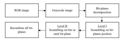
Figure 2: Block diagram of image scrambling
