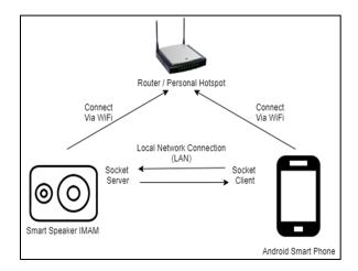
Figure 3. IMAM Smart speaker with outer and smartphone
