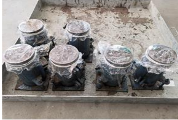
Figure 4. The mould is covered with thin plastic sheet wrap to prevent moisture loss
