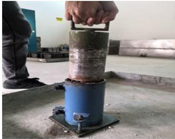
Figure 3. Mix of porous concrete compacted with compaction weight
