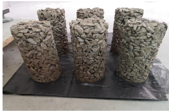
Figure 5. Geopolymer porous concrete specimens
