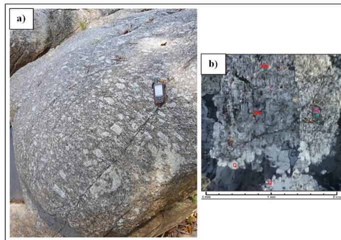
**Figure 7.** a) Granite outcrop and b) photomicrograph of alkali feldspar granite (Q=Quartz, Kfs=Alkali Feldspar).
