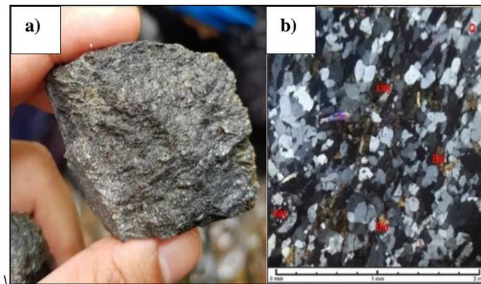
**Figure 2.** a) Schist sample, b) photomicrograph of schist (Q=Quartz, Bio=Biotite).
