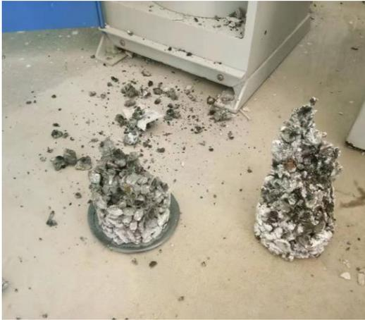
**Figure 21.** Crushed porous concrete (PC4)
