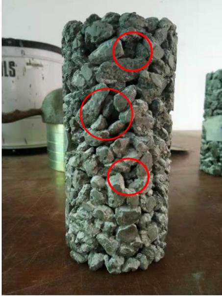
**Figure 17.** Porous concrete with large voids (PC3)
