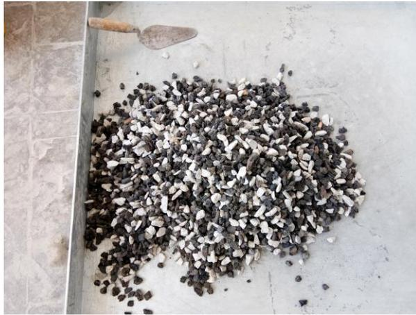
**Figure 2.** Bottom Ash and Normal Aggregates mixed manually on a pan
