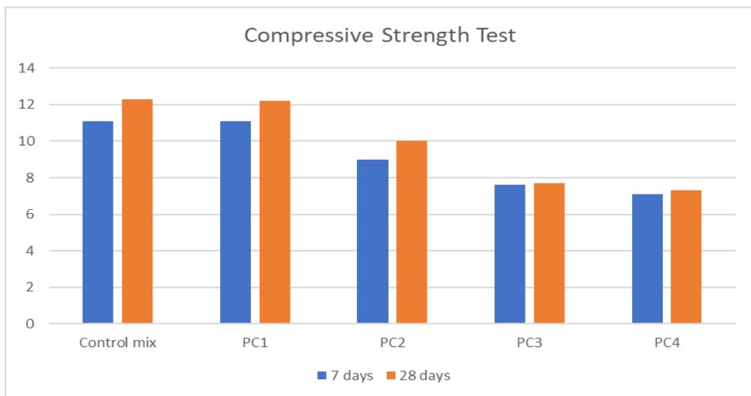
**Figure 12.** Chart of compressive strength test of porous concrete
