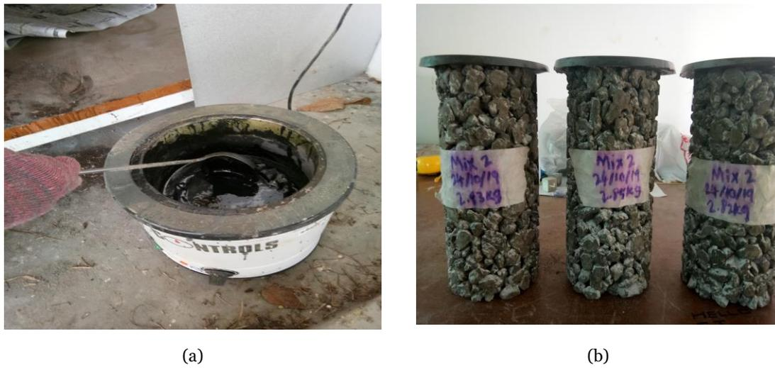
**Figure 4.** (a) Sulphur heating, and (b) Porous concrete capped with sulphur
