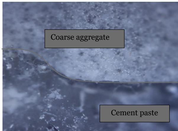
**Figure 23.** Bonding of coarse aggregate with cement paste
