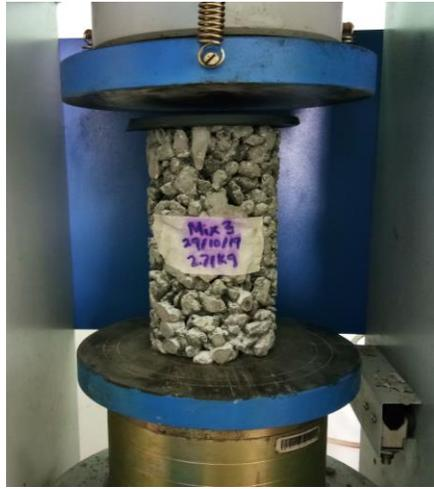
**Figure 7.** Compressive strength test
