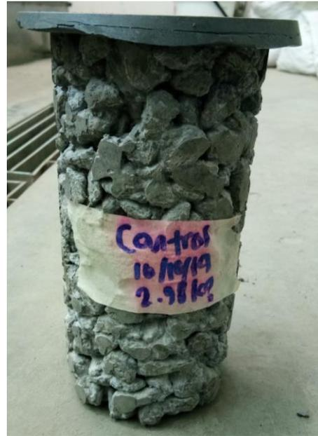
**Figure 22.** Intact normal porous concrete after compressive test
