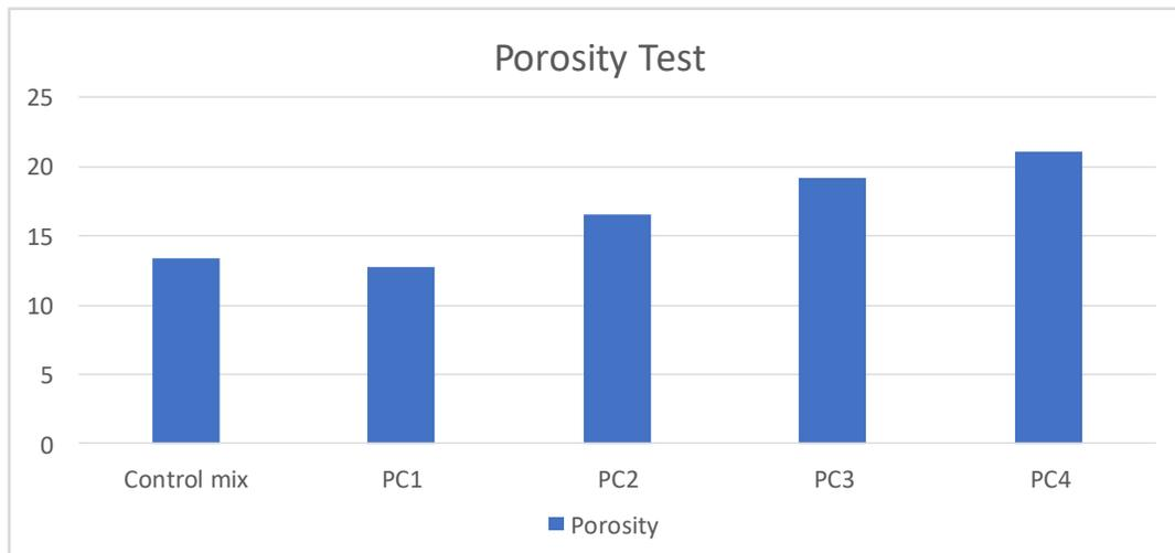
**Figure 9.** Porosity of porous concrete
