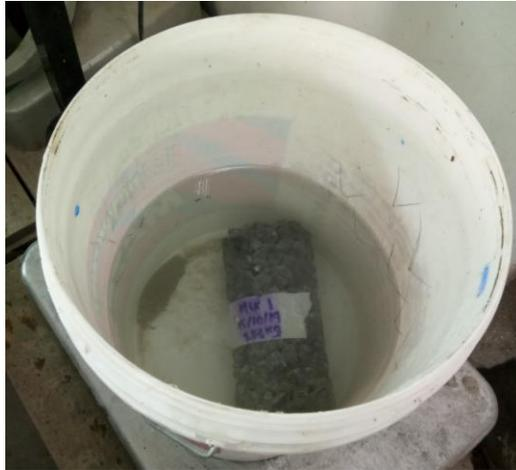
**Figure 5.** Porosity test
