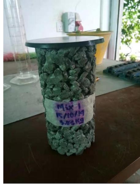
**Figure 18.** Well compaction of porous concrete
