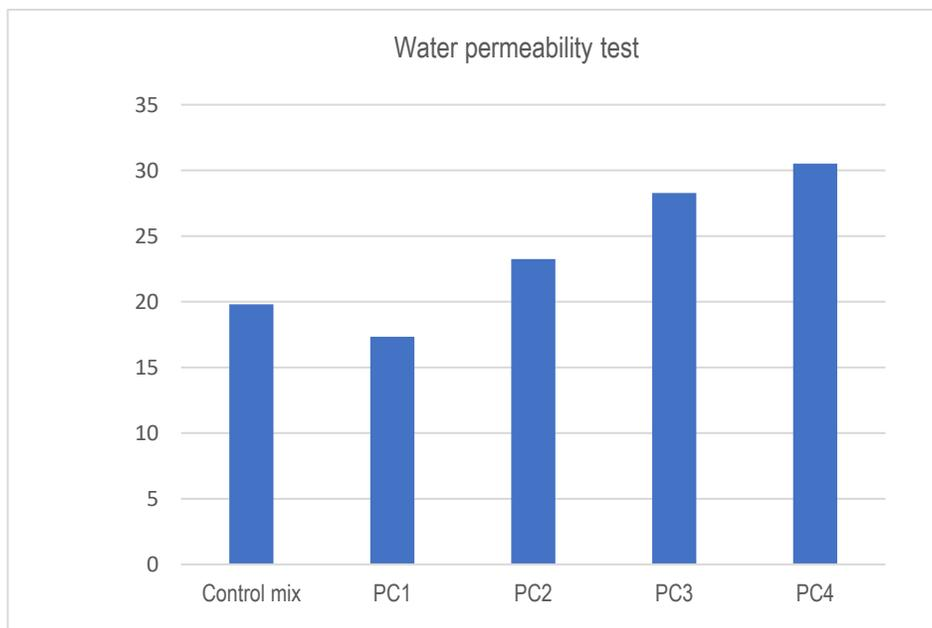
**Figure 11.** Chart of water permeability of porous concrete
