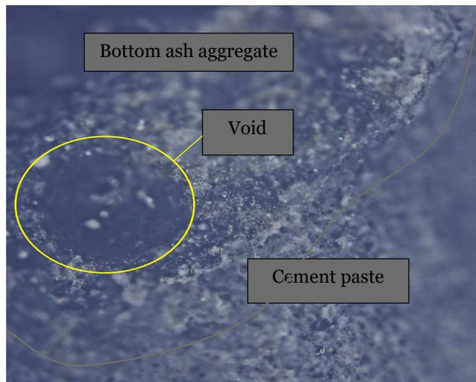
**Figure 24:** Bonding of bottom ash aggregate with cement paste
