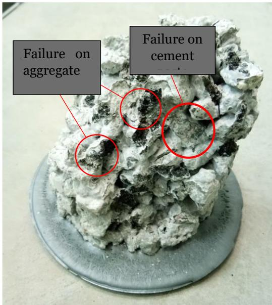
**Figure 19.** Failure of bottom ash aggregates (PC4)
