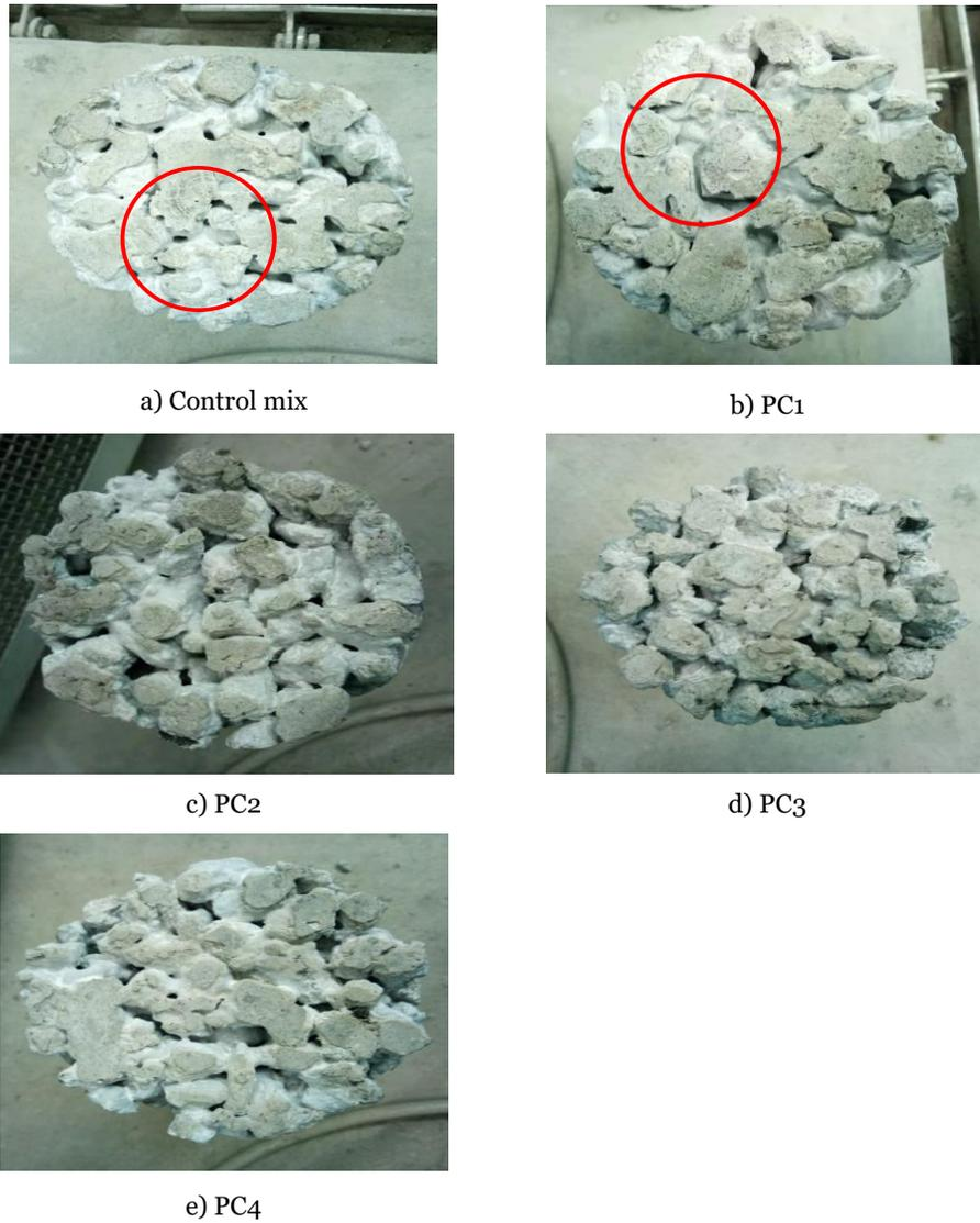
**Figure 10.** Binder Paste and Aggregates: a) NPC, b) PC1, c) PC2, d) PC3 and e) PC4
