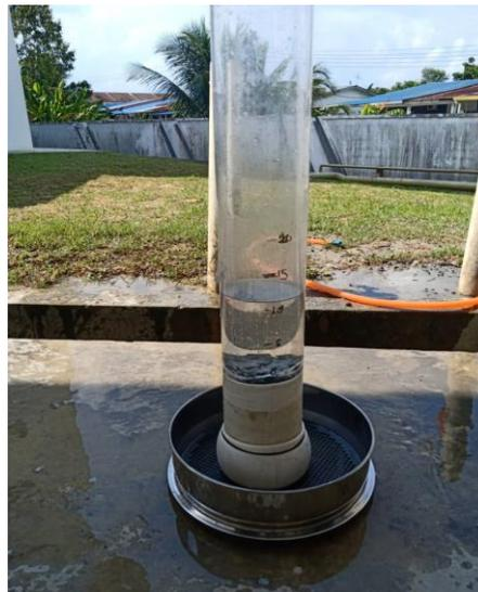
**Figure 6.** Water permeability set-up
