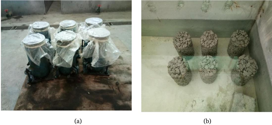
**Figure 3.** (a) Moulds covered with with cling wrap, and (b) Water curing
