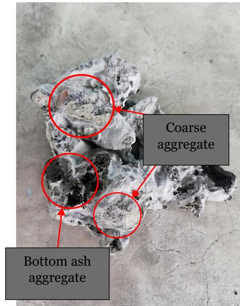
**Figure 20.** Piece of crushed concrete
