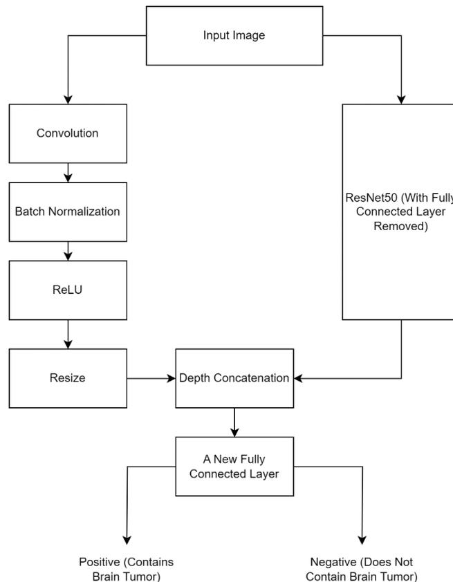
**Figure 3.** The proposed model (modified ResNet50).
