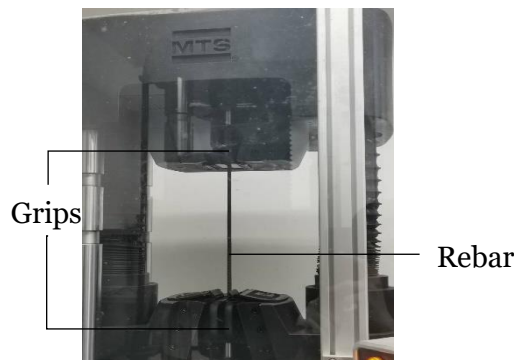
Figure 9. Tensile Test of Rebar
