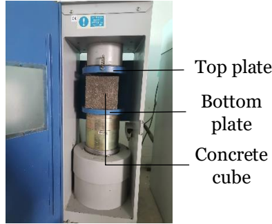
Figure 8. Concrete Cube Test
