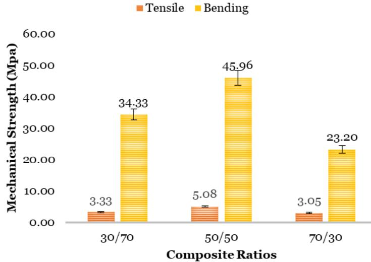
**Figure 2.** Bending and flexural strength for LDPE/bamboo fiber composite
