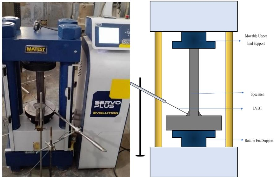
**Figure 5.** Test arrangement of the square steel section T-joints with schematic view.
