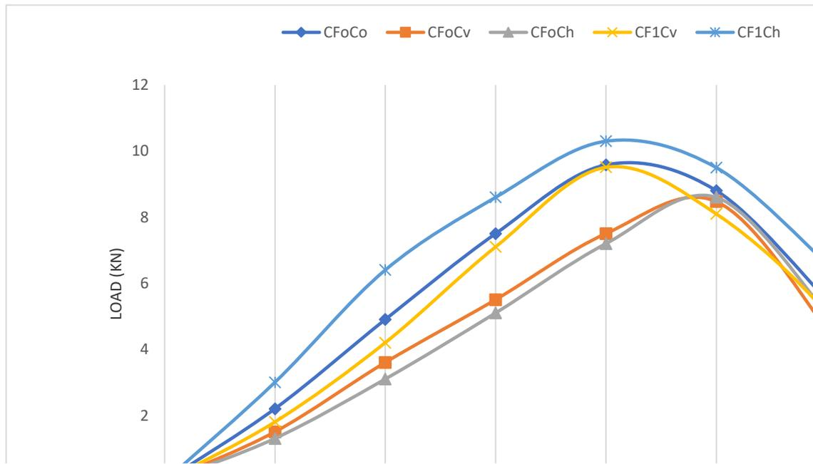
**Figure 7.** Load vs Displacement (C-joint)
