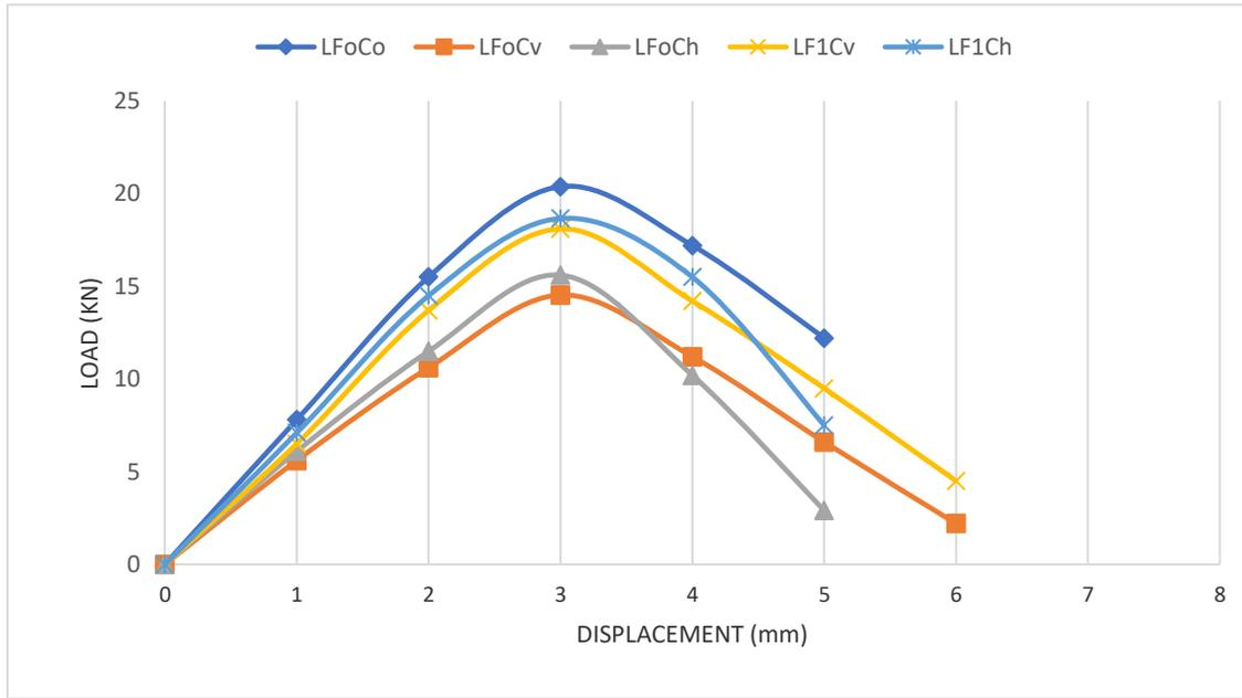
**Figure 8.** Load vs Displacement (L-joint)
