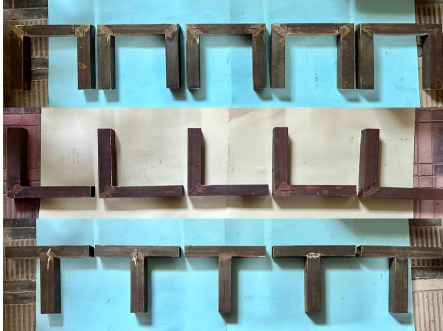
**Figure 4.** Square section C, L & T-joint specimen
