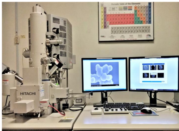
Figure 1. The FESEM and instrument that was used to examine the morphology of carbon nanoparticles [8].
