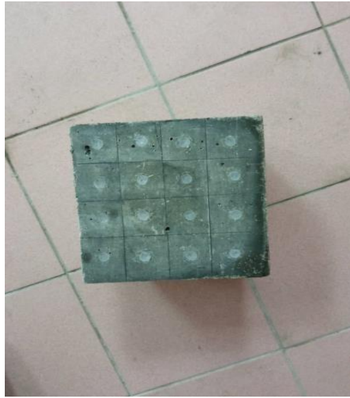
Figure 12. Marked position for rebound hammer test
