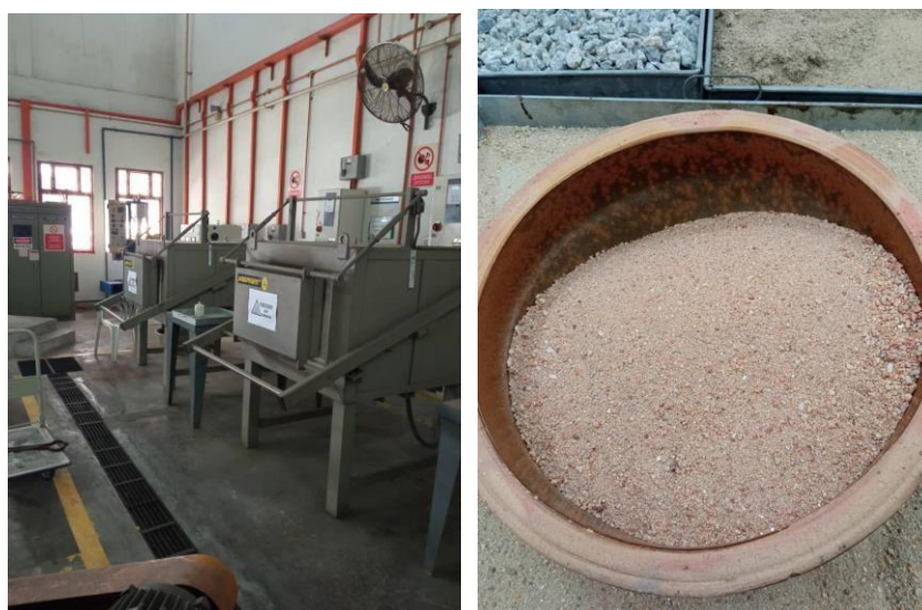
Figure 6. Calcination process in the furnace (left) and calcined dredged sediment (right)
