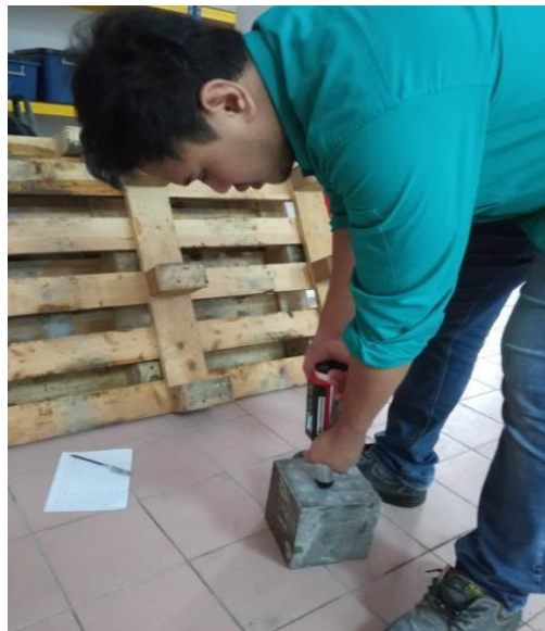
Figure 13. Rebound hammer test procedure
