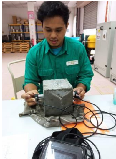
Figure 11. UPV test procedure
